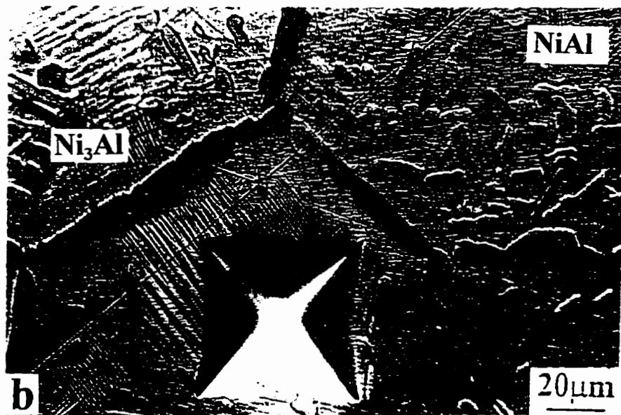
Figure 3.8 Typical micrographs of Vickers microhardness testing on (a) the "mat-structure" of the aged \text{Ni}_{65.9}\text{Al}_{34.1} ( 1000^\circ/100\text{h} + 500^\circ\text{C}/100\text{h} both followed by a slow furnace cooling), and (b) the twin-structure of the homogenized \text{Ni}_{63.7}\text{Al}_{36.3} ( 1000^\circ/100\text{h} followed by a slow furnace cooling) in-situ composites under 2000g load.
