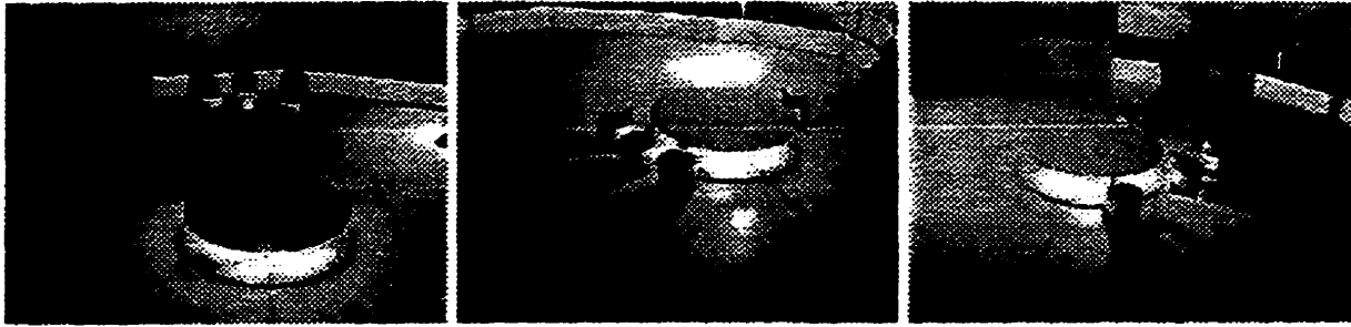
Figure 6.9: Shown are five robots pushing a round box from its initial position first towards a goal-light in the right of the picture and then towards a goal-light on the left of the picture. The mpeg video from which this sequence was taken is available at http://www.cs.ualberta.ca/~kube/
