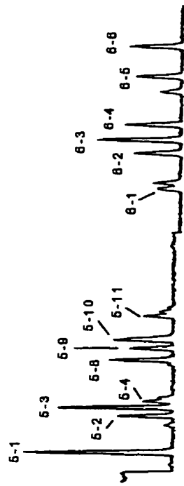
Figure 2. GC-NIMS chromatograms of technical PCN standard (Halowax 1014) and an air sample from Alert. The 5/6-CI section of the chromatogram in the Alert sample is magnified by a factor of ten. Peak labelling and identification is presented in Harner and Bidleman (1997).
