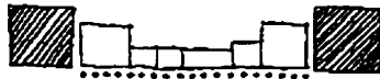
3. Parking lots and anchor stores are at the ends of the linear arrangement.
