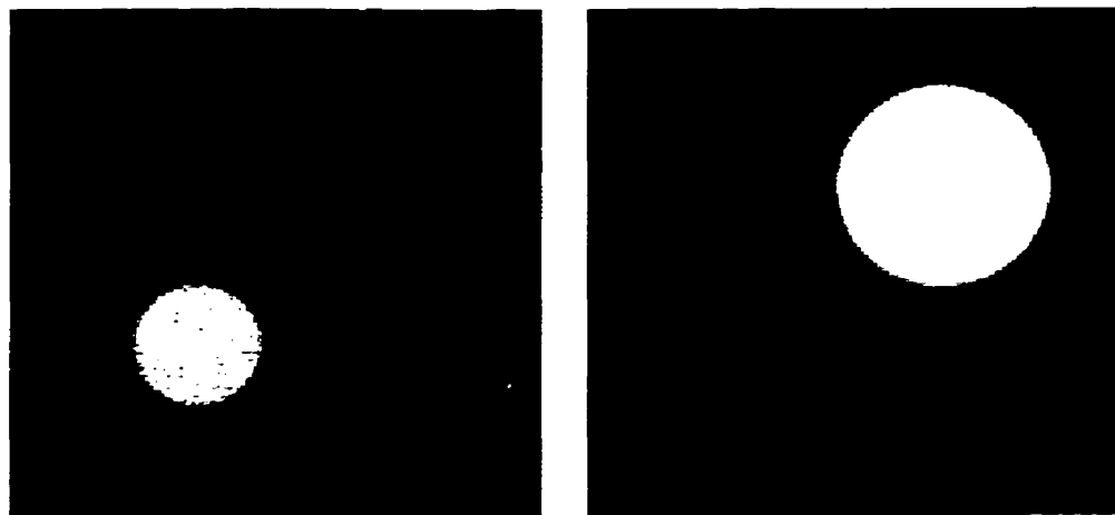
Figure 5.2: Isolated T_2 species from two RARE-mode acquisitions The image on the left is the isolated T_2=40\text{ms} disk phantom of diameter 25% of the FOV, and that on the right is the T_2=120\text{ms} disk phantom. The images are normalized to unity at the brightest pixel, and both images are at the same windowing level.
