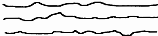
Figure 2.2: A schematic diagram showing the possible roughness of interfaces in a superlattice in contrast to the purely one-dimensional structure as shown in figure 1.1
